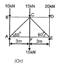
(b) Determine the magnitude and nature of forces in the members of truss as shown in figure by Graphical method.
