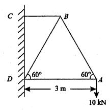
(d) Determine the magnitude and nature of forces in the members of truss as shown in fig. by method of joints.
